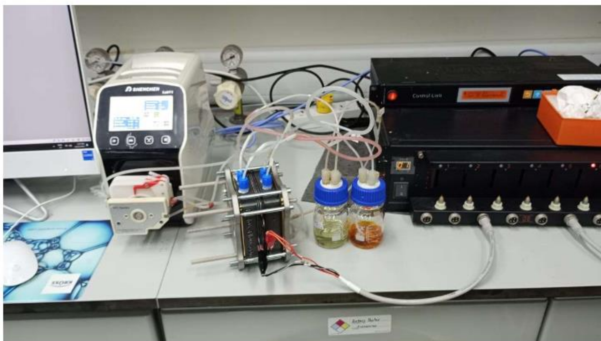
Fig 2: AORFB testing experimental setup, displaying electrolyte tanks, pumps, tubing, flow cell, and monitoring apparatus.
