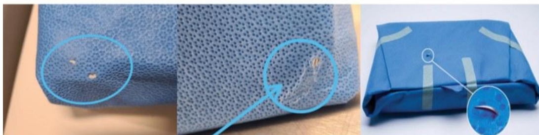
Figure 1.5: Three examples of punctured and torn SMS non-woven wrap. Left and centre: close-up views showing small puncture holes (circled in blue). Right: intact-appearing pack with a close-up inset revealing a needle tip protruding through the
