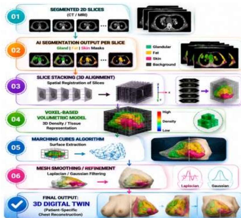
Figure 3: demonstrates the transformation from segmented slices to volumetric 3D reconstruction and mesh generation
